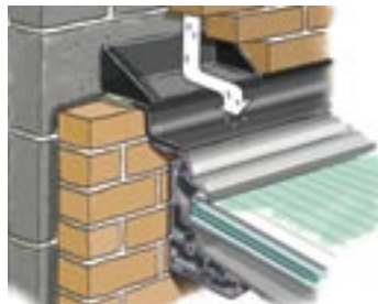
How cavity trays prevent water penetration
